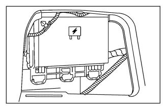
The rear compartment fuse block is located in the trunk of the vehicle. Access the fuse block through the trunk panel on the driver's side of the rear cargo area.
